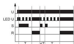
The input of the time relay is supplied with voltage U continuously. Closing of the control contact S starts the interval T, and after the interval T has lapsed, the output relay R switches on and remains in this position until the control contact S is closed again or until the supply voltage U is interrupted. Closing of the control contact S resets the thus far measured time and starts the new interval T.
