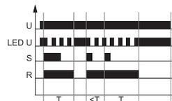
The input of the time relay is supplied with voltage U continuously. Closing of the control contact S immediately switches the output relay R on for the set interval T. After the interval T has lapsed, the output relay R is switched off. The next closing of the control contact S immediately switches on the output relay R for the interval T. In case the control contact S is closed within the interval T, the measured time is cancelled, and the interval T starts again.
