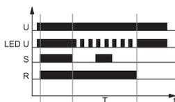
The input of the time relay is supplied with voltage U continuously. Closing of the control contact S immediately switches on the output relay R. Opening of the control contact S starts the set time of the delayed switching off of the output relay R. After the interval T has lapsed, the output relay R switches off. Opening or closing of the control contact S within the interval T does not affect the function to be performed.
