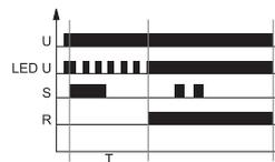
The input of the time relay is supplied with voltage U continuously. Closing of the control contact S starts the interval T, and after the interval T has lapsed, the output relay R switches on and remains in this position until the supply voltage U is interrupted. When the output relay R is on, opening or closing of the control contact S does not affect its status.
