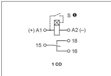
① The control terminal S is activated by connection to A1 terminal via the external control contact S.
