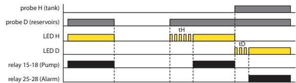
The relay is designed to monitor the level of conductive liquids with a choice of 8 functions:
